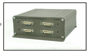
Medium configuration cameras are supported using two CLM-601s in parallel. Multiple CLM-601s may be cascaded to support more than four cameras.
