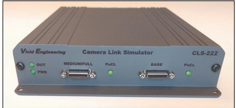
enhanced timing performance, bayer color support, and color bar & pseudo-random video patterns. Control is via an RS-232 port, USB, or frame grabber comm port. The CLS-222 also supports the AIA validation test pattern.
