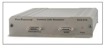
The CLS-212 is controlled using a PC with a standard RS-232 serial port, or USB port using an optional adapter. CLS-212 control is performed via a simple, straightforward, Command Line Interface (CLI). No special software is required. Configuration files are easily created with user parameters and downloaded to the CLS-212.
