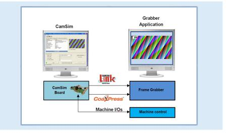
The Gidel **CamSim™** is a flexible high-performance camera simulator that generates CoaXPress and camera link video stream and test patterns for testing frame grabbers or vision/imaging systems. The system supports all CoaXPress v1.1 and Camera Link<sup>™</sup> v2.0 configurations and can be customized for any user-defined camera protocol and interface.
