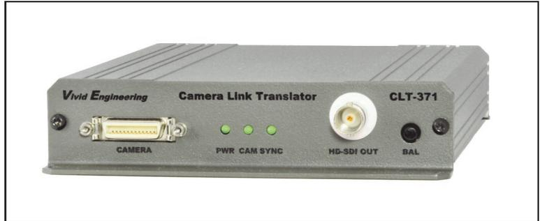
Features include automatic frame rate adaptation, Bayer white balance correction, camera synchronization support, and an RS-232 port for camera set-up and control.
