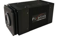
A key feature of the IMX420 Sony sensor is a Dual ADC mode, where each pixel can be read out with two different gains. The PL-X957 combines the Dual ADC images into a single hybrid HDR image, directly on camera - thus removing the need for any host processing. Real time on camera HDR is an easy way for the user to gain 6-10dB of additional dynamic range on their image without taxing the CPU or requiring additional complex software algorithms.
